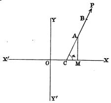
If a, b, a, P be given, it is clear that the force is completely determined; for a, b, determine its point of application A, a determines its direction and P its magnitude.
